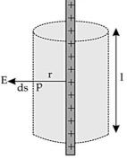
(a) Electric field due to an infinitely long straight wire having uniform linear charge density  $\lambda$ : x = Distance of the point P from the wire where the electric field is to be evaluated
