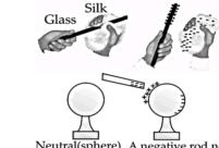
Neutral(sphere) A negative rod near by separates +ve and -ve charges
