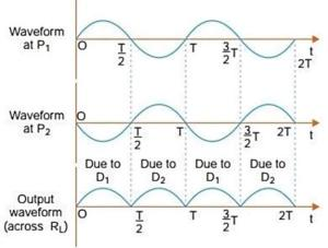
In a full wave rectifier, if input frequency is f hertz, then output frequency will be 2f hertz because for each cycle of input, two positive half cycles of output are obtained.
