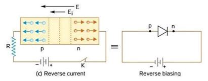
When the potential difference across the junction is increased in steps, a very small reverse current of the order to micro-amperes flows. The reason is that due to thermal agitation some covalent bonds of pure semi-conductor break releasing a few holes in n-region and a few electrons in p-region called the *minority charge carriers*. The reverse bias opposes the majority charge carriers but aids the minority charge carriers to move across the junction. Hence a very small current flows.
