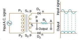
flows in diode  $D_2$  and there is no current in diode  $D_1$ . The direction of current  $i_2$  due to diode  $D_2$  in load resistance is again from A to B Thus, for input ac signal the output current is a continuous series of unidirectional pulses. The input and output sequels are shown in the figure. This output current can be converted into steady current by the use of suitable filters.
