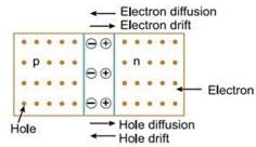
In same way, electrons on the n-side are close to the junction plane tend to diffuse across it and into the p-side, where there are very few free electrons. Similarly, holes on the p-side are close to the junction plane tend to diffuse across that plane and into the n-side, where there are very few holes. The motions of both the electrons and the holes contribute to a diffusion current  $(I_{\text{diff}})$ .
