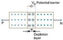
**Potential barrier:** During the formation of a p-n junction the electrons diffuse from n-region to p-region and holes diffuse from p-region to n-region. This forms recombination of charge carriers. In this process immobile positive ions are collected at a junction toward n-region and negative ions at a junction toward p-region. This causes a potential difference across the unbiased junction. This is called potential barrier.
