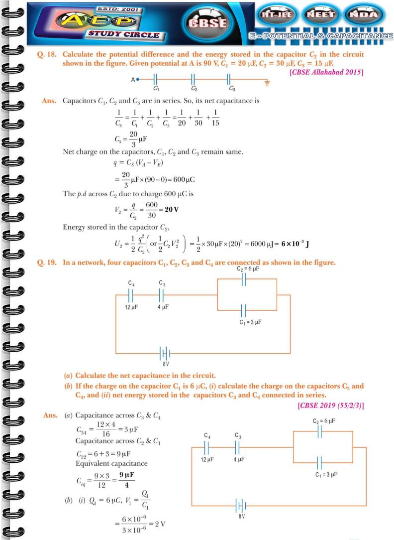
Q. 18. Calculate the potential difference and the energy stored in the capacitor  $C_2$  in the circuit shown in the figure. Given potential at A is 90 V,  $C_1 = 20 \mu F$ ,  $C_2 = 30 \mu F$ ,  $C_3 = 15 \mu F$ .
