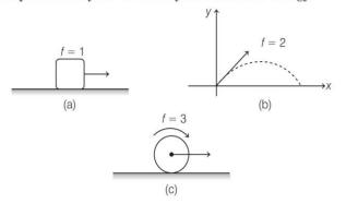
**For example** In Fig. (a), block has one degree of freedom, because it is confined to move in a straight line and has only one translational degree of freedom.
