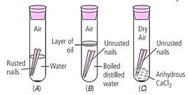
**Observations**: Only in test tube A, iron nails get rusted since the nails in this test tube are exposed to both air and water.
