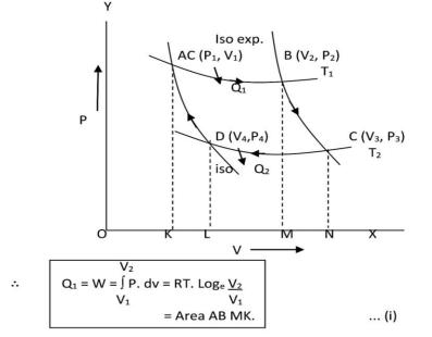
—Stage (2): Adiabatic Expansion: The cylinder is now removed from the source and is placed on the perfectly insulating pad. The gas is allowed to expand further from B (V<sub>2</sub>. P<sub>2</sub>) to C (V<sub>3</sub>, P<sub>3</sub>). Since the gas is thermally insulated from all sides, no heat can be gained from the surrounding temperature of gas falls to T<sub>2</sub>, the expansion is adiabatic (represented by curve BC)
