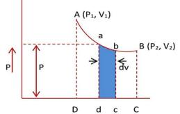
Consider two point 'a' & 'b' on P-V diagram. The point 'a' & 'b' are so closed to each other that the pressure 'P' corresponding to these points is same. Now we have to draw 'ad' & 'bc',  $\perp^{r}$  on the volume axis. Here dc = dv (change in volume).
