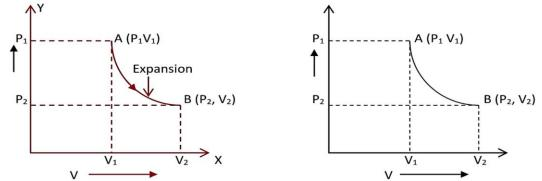
Consider 1 mole of gas in a cylinder filled with a frictionless piston. Let gas expends from the state A ( $P_1$ ,  $V_1$ ) to the state B ( $P_2$ ,  $V_2$ ).
