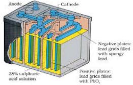
When the battery is in use, the following cell reactions take place:
